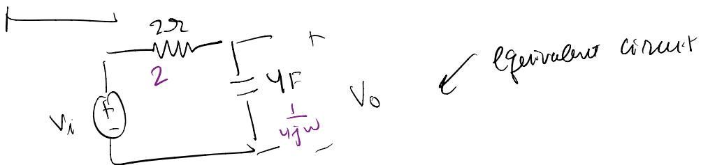
Voltage divider:  $V_o = \frac{\frac{1}{4j\omega}}{2 + \frac{1}{4j\omega}} V_i$
