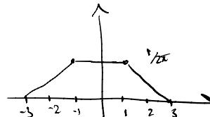
(5) Suppose  $F(\omega)$  is as shown below. What is its inverse Fourier transform  $f(t)$ ?
